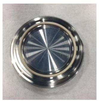
Place the quartz disc, PD183-07, on top of the chamber base.
