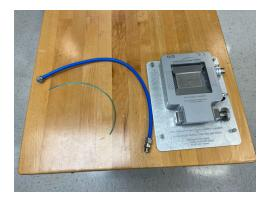
To connect a vacuum pump, use a 5/8" socket wrench to remove the cap on one of the two accessory ports on the side of the chamber.
