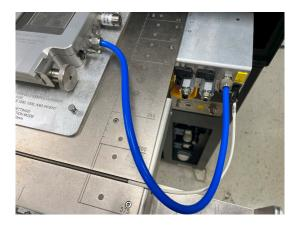
Then connect the vacuum pump directly to vacuum port on the PulseForge® sample table interface and make sure the vacuum pump is plugged into an outlet. The vacuum pump can be run without the introduction of gas to create a vacuum environment. Be aware that depending on the pump and hosing configuration, the maximum vacuum will be in mTorr range.
