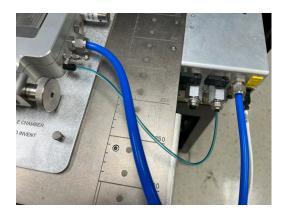
If desired, both the vacuum and gas can be engaged simultaneously to remove any oxidizers from the process environment. The pressure inside the chamber can be adjusted using the needle valve on the input.
