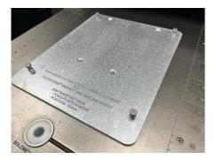
4. Line the pins on the bottom of the chamber up with the fixture plate and it will click as it is seated in place.
