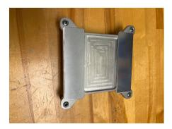
7. Place the sample in the chamber and secure it using the two magnetic hold-down strips.
