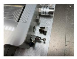
Connect the vacuum hosing from the accessory port to the associated port on the side of the PulseForge® sample table.
