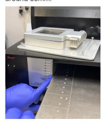
3. Once the sample table is at the appropriate height, line up the four spring pins on the fixture plate with the holes in the center of the sample table. They will snap into place.
