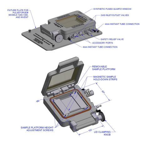
**Fixture Plate:** Provided for mounting to the sample stage on PulseForge Models 1200, 1300, and Invent curing systems.
