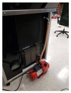
10. With the external vacuum pump, a more precise vacuum gauge is needed. The following image shows how the vacuum line should be connected to the chuck. The pressure gauge is turned on by pushing and holding the blue button in the center. The pressure read out is in mTorr. The operation of the tool is as previously stated.
