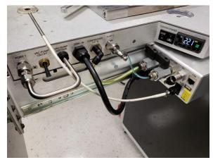
5. Vacuum is pulled by turning on the small pump in the vacuum chuck housing (small switch marked "VAC PUMP ON/OFF"). The vacuum is pulled through the porous graphite chuck. This enables attachment of the product piece to the graphite plate for improved thermal contact. If desired, the inert gas could be turned on at the same time to provide an inert processing atmosphere. The inert gas enters the chamber through the port 2 hole in the bottom right corner of the graphite plate.
