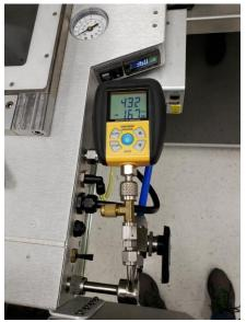
11. There is a brass purge valve on the side of the vacuum gauge. This purge valve is used to repressurize the sample chamber. First close the black vacuum valve and then turn the purge knob to repressurize the sample chamber
